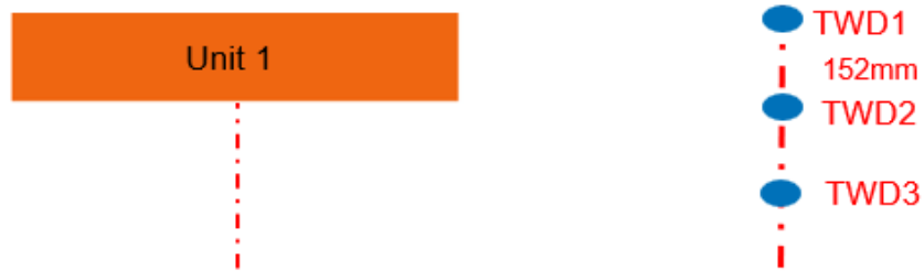
Figure 12. Vertical positions of the thermocouples on the wall D
