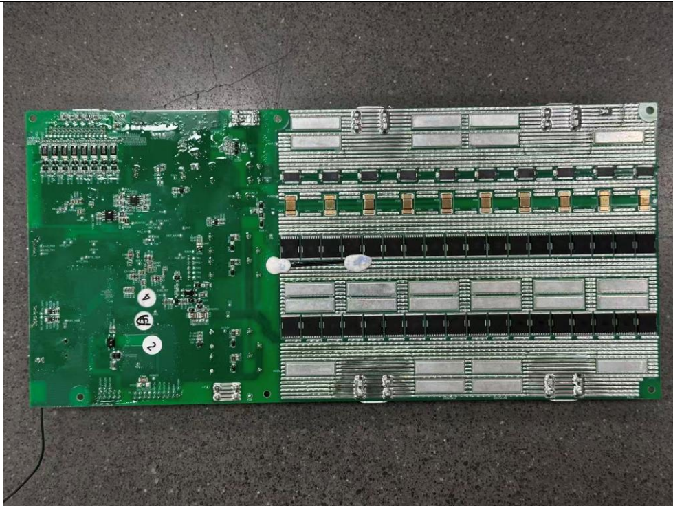
Back view of BMS board
